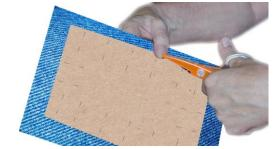
Ensure template is secured to fabric to allow for accuracy. Double sided tape can be used instead of pins to do this.
